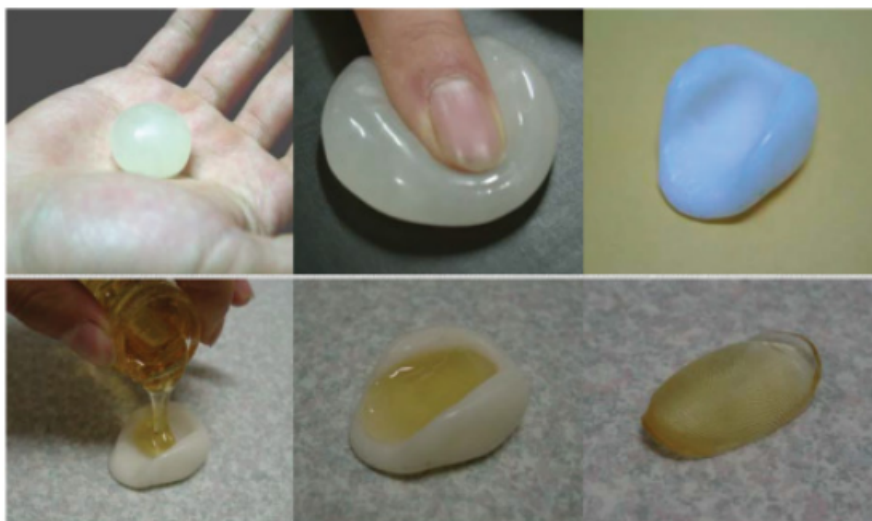
Figure 2.7: Steps of spooft making in a cooperative mode from [Marasco and Ross, 2014], originally from Matsumoto http://web.mit.edu/6.857/OldStuff/Fall103/ref/gummy-slides.pdf
